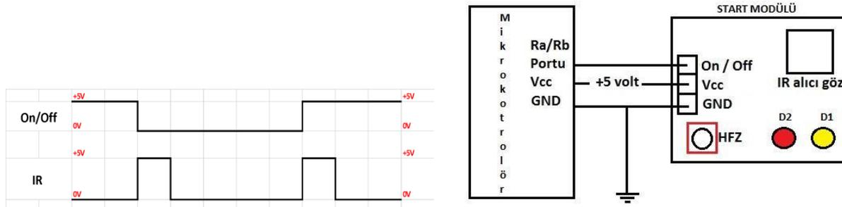
**Figure 6** Wiring diagram between MCU and start module
