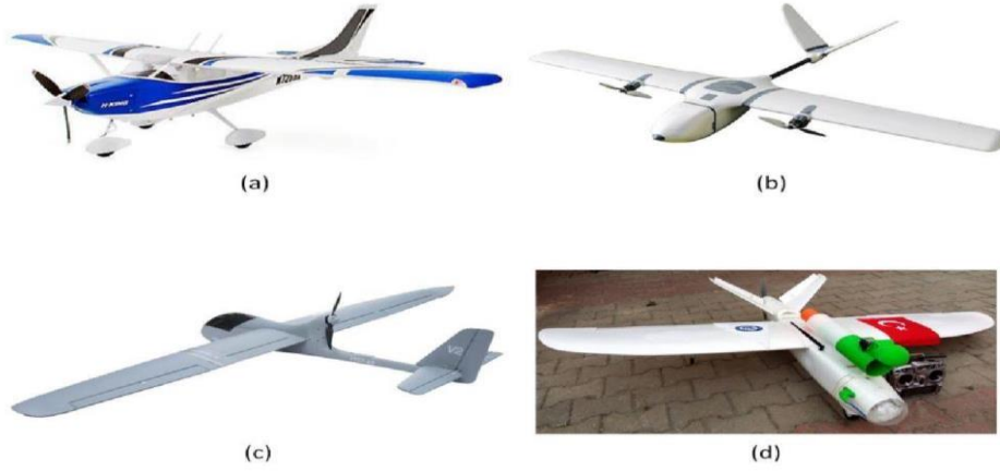
Figure 1: Fixed Wing UAV Images: Front Motorised (a), Wing Motorised (b), Top Motorised (c) and Rear Propulsion (d)
