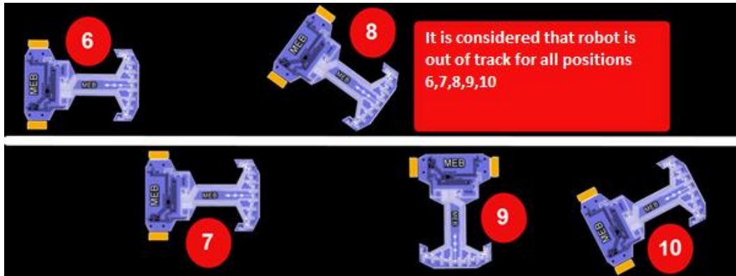
Figure 7: Positions of robot on the track
