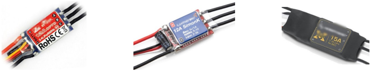
Figure 8. Drone motor drivers.
